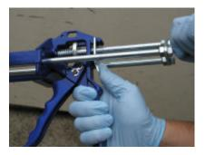
Insert twin tubes into the caulking gun, making sure the bottom of the tubes line up with the twin plungers. Do not pull trigger or snug the plungers up to the tubes at this point.
