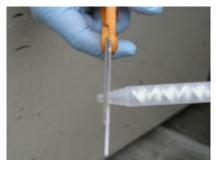
Note: A 1/4" bead is sufficient for most caulking jobs. Large gaps between the island forms and the concrete will require a thicker bead. Simply cut the tip of the mixing nozzle at the third or fourth shoulder in order to fill the larger gaps. Be sure you use enough paste to adhere to both the island form and the concrete.
