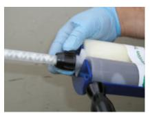
10. At the tip of each mixing nozzle, there are several ridges or shoulders. Using a utility knife, score around the second shoulder from the tip and carefully cut the tip off at this point for a ¼" bead. Do not cut the tip at an angle. Take care, as the plastic mixing nozzles are sturdy and difficult to cut.
