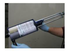
8. Remove the threaded collar and the half-moon plugs from the tips of both tubes and save.
